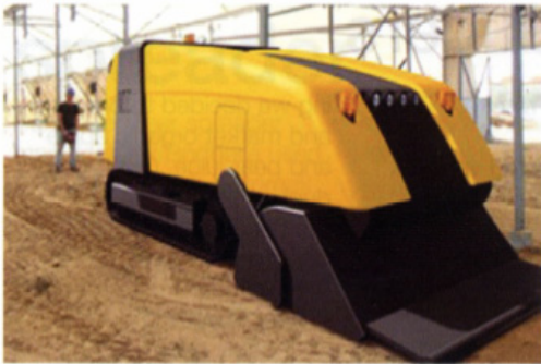
The Cultivit heats soil to 800 degrees at a depth of 35cm.
